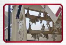
Twin webs allow for material to be fed out the 62" wide opening and into the same 18" horizontal beaters as the larger machines use. From there the spinners spread your material evenly across the pattern. Bridging is impossible...
